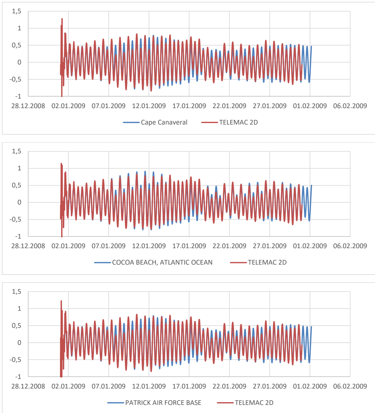
Fig. 83: Comparison of water levels predicted by the model and by the NOAA tidal predictions at Cape Canaveral, Cocoa Beach and Patrick Airforce Base.
